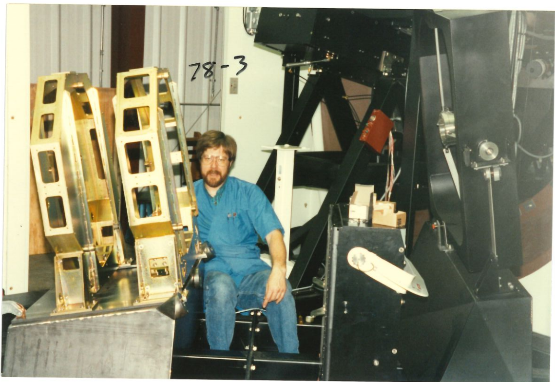
Alignment check with the empty lens cells. Jim Ward is adjusting (78-1, -3)
