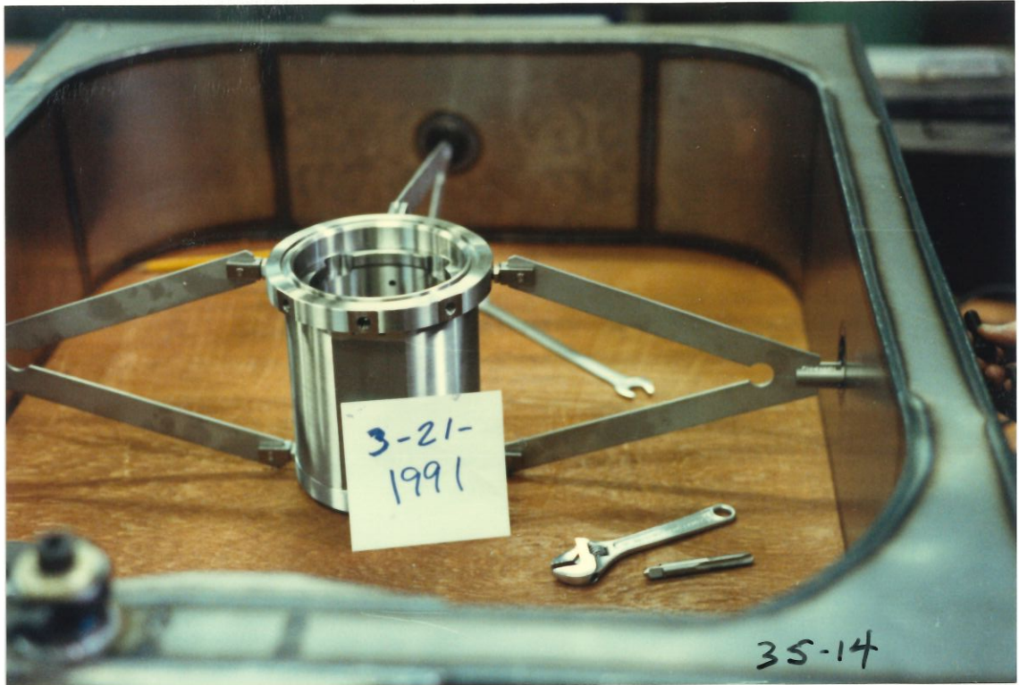
Spiders at initial installation and centering. (35-14)
