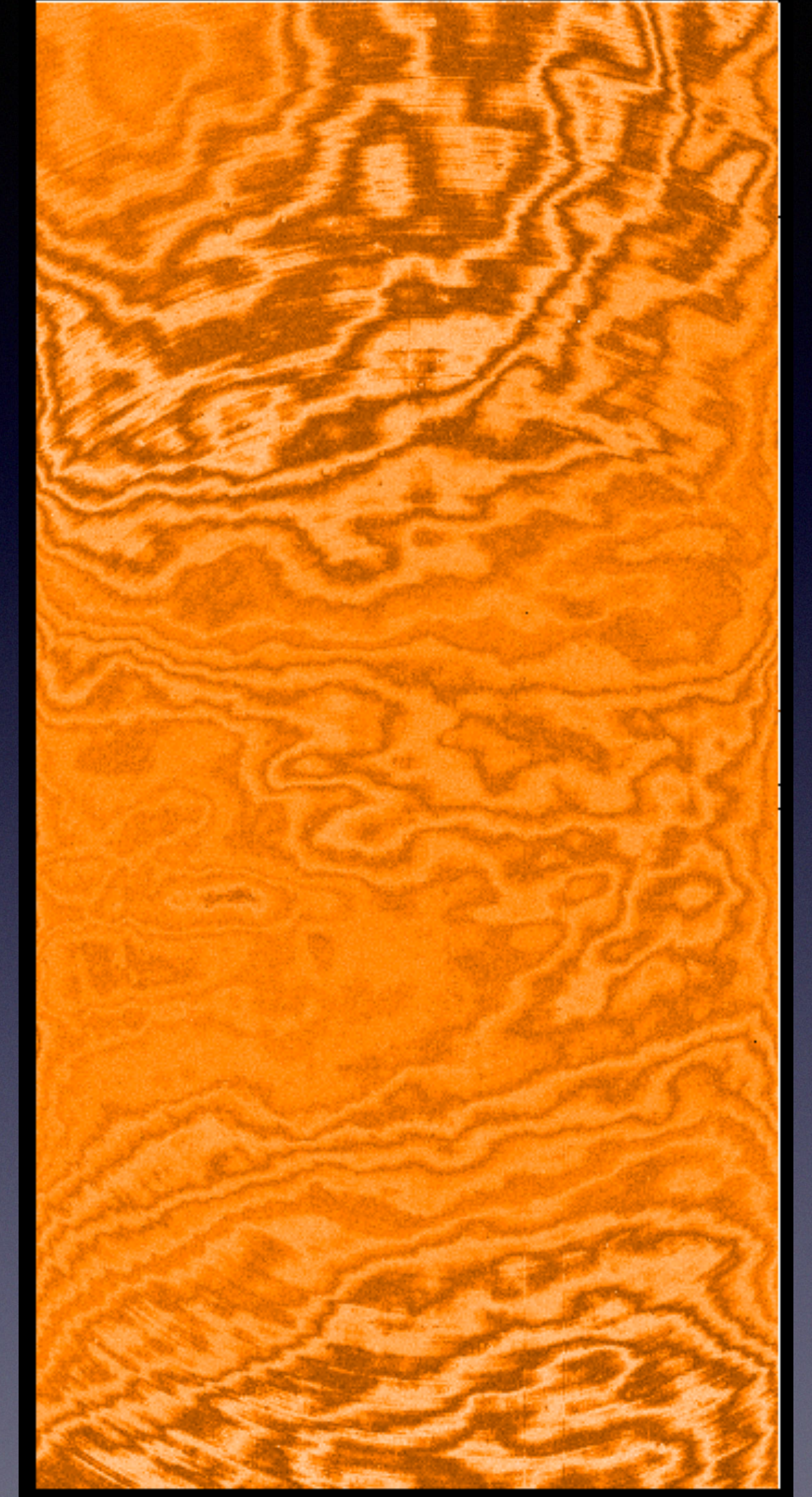
Example Z-band fringe frame for INT-WFC
